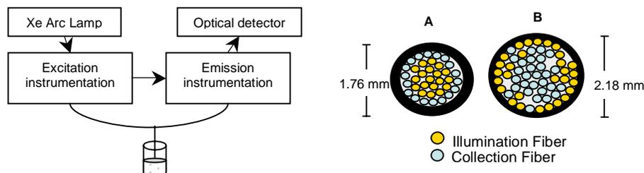
Fig. 1. (a) Generalized schematic of the instruments used; (b) Schematic of probes A and B
