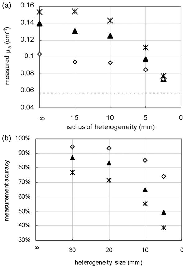
Fig. 5. (a) Measured absorption coefficient ( $\mu_a$ ) of a tissue phantom containing a heterogeneity and (b) measurement accuracy for data presented in (a). The values of  $\mu_a$  of the heterogeneities are ( $\star$ ) 0.20 cm<sup>-1</sup>, ( $\blacktriangle$ ) 0.15 cm<sup>-1</sup>, and ( $\diamond$ ) 0.10 cm<sup>-1</sup>. The dashed line in (a) represents the measured  $\mu_a$  of the background. The reduced scattering coefficient ( $\mu_s'$ ) of the entire phantom is 10 cm<sup>-1</sup>.
