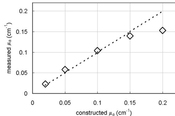
Fig. 3. The measured (diamonds) and theoretical (dashed line) absorption coefficient ( $\mu_a$ ) of the homogeneous agar phantoms for  $\mu_a$  from 0.02 to 0.20  $\text{cm}^{-1}$  and for a value of  $\mu_s'$  of 10  $\text{cm}^{-1}$ .
