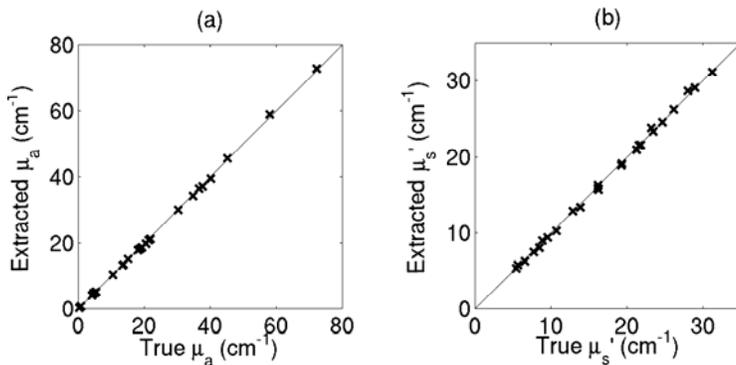
Figure 1: Scatter plots of the extracted vs. expected optical properties for the (a) absorption coefficient and (b) reduced scattering coefficient. The solid line is the line of perfect agreement. These results are for the fiber design with 2 collection fibers.
