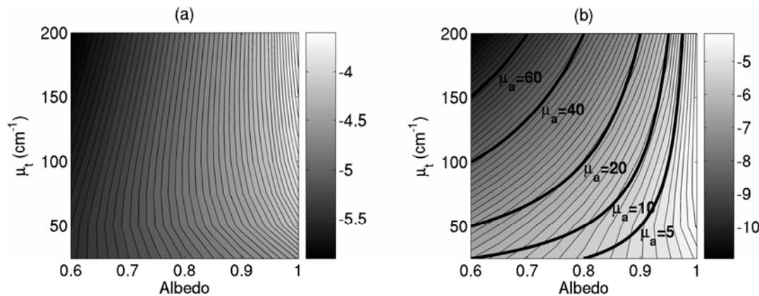
Figure 2: Log contour plots of the collected diffuse reflectance from (a) fiber 1 and (b) fiber 2. It can be seen that the contour lines in (a) roughly follow the vertical lines of equal albedo, while the contour lines in (b) roughly follow the lines of equal  $\mu_a$  (bold lines).
